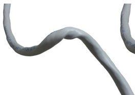
Cable kinks should be replaced
